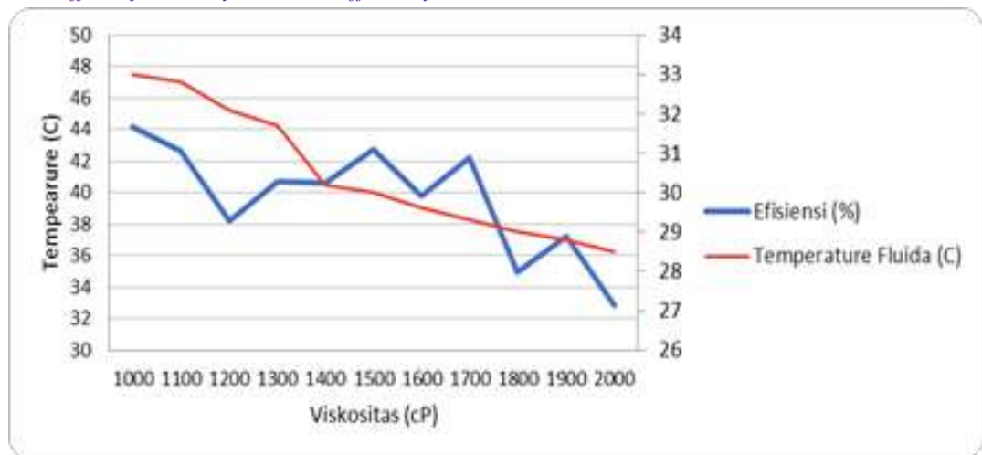
Figure 15. Effect Viscosity on Motor Efficiency
