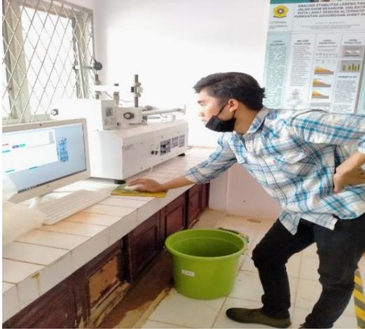
**Gambar 2.** Pengecekan proses uji geser langsung (*direct shear*).
