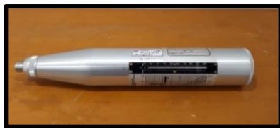
Gambar 6. Alat Uji Hammer Test
