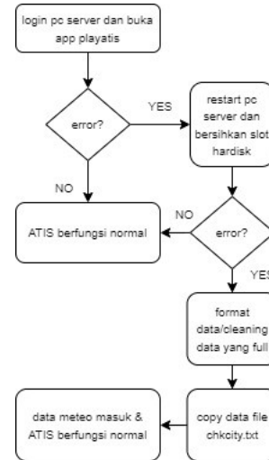
Gambar 1. Flowchart proses corrective maintenance ATIS
