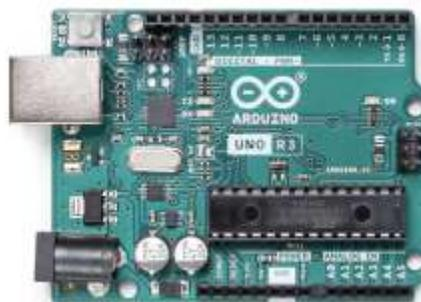
Gambar 6. *Board* Arduino Uno (Sumber: <https://store.arduino.cc/products/arduino-uno-rev3>)
