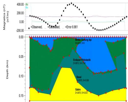
Figure 10. Model slice C-C' from Slice Map Reduction to Pole
