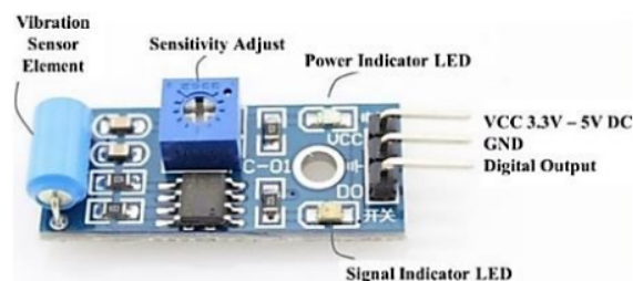
Figure 2. SW-420 sensor module
