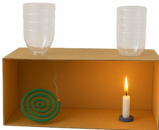
Figure 2 Simple Convection Tube
