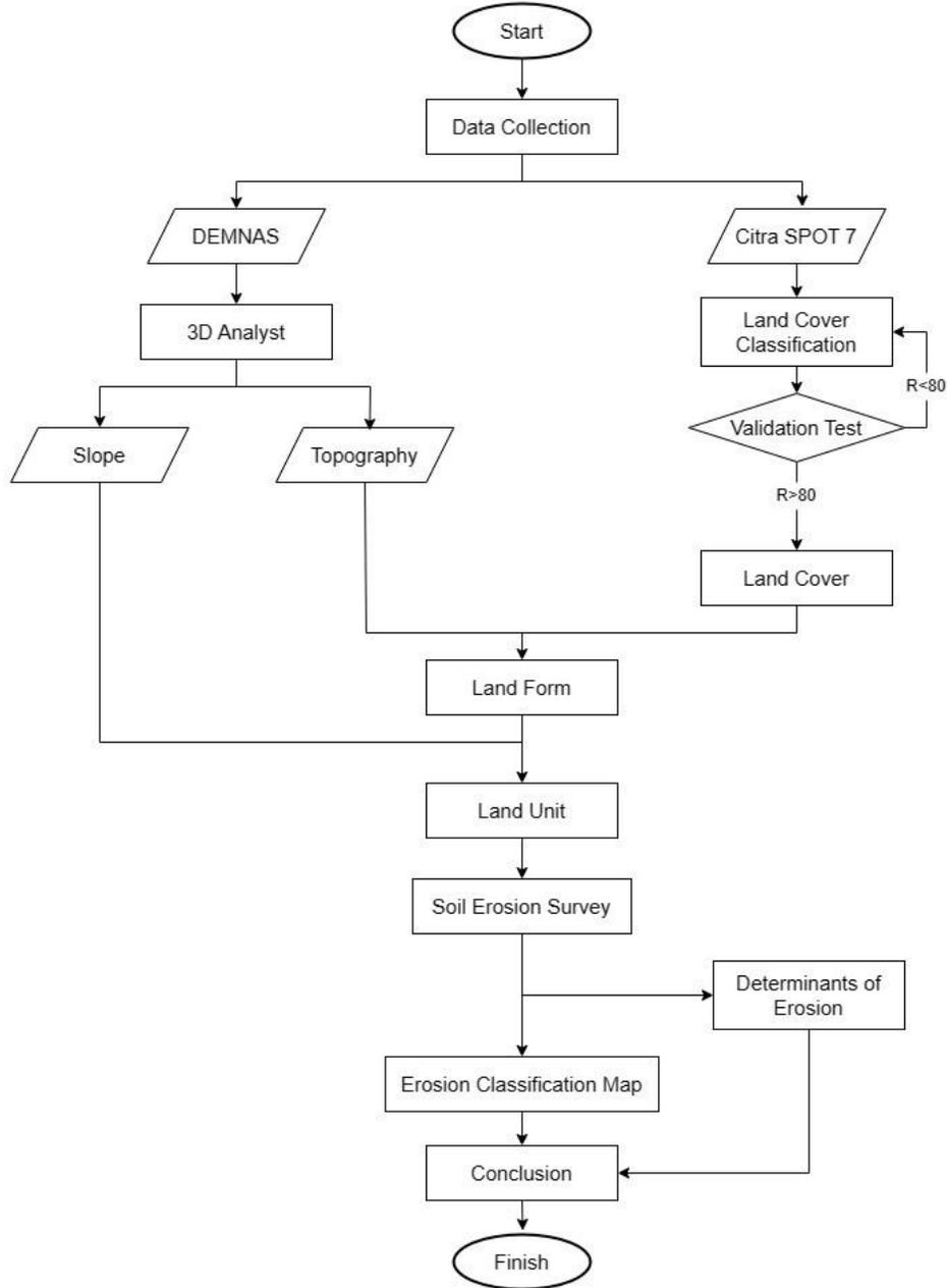
**Figure 2.** Research Flow Diagram
