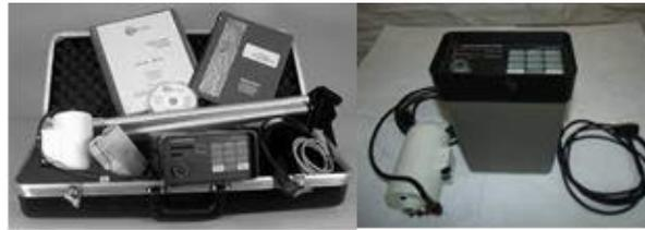
Gambar 2. Alat PPM (Proton Precession Magnetometer)
