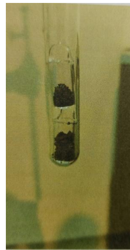
Gambar 9. Serbuk hasil proses hydride-dehydride (Author's)
