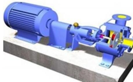
**Gambar 3.** Pompa Sentrifugal [2].
