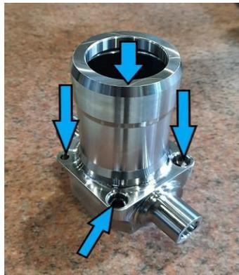
**Gambar 18.** *Finishholes, face mill and drive dog removal*
