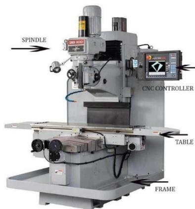
**Gambar 3.** Bagian-Bagian Mesin Milling CNC
