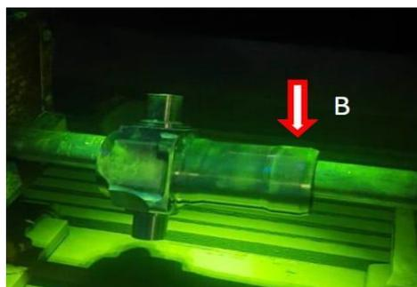
**Gambar 19.** *Magnetizing flaw detect*
