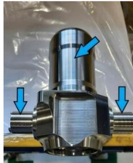
**Gambar 14.** Turnmill finish turn, second side. trunnion mill finish
