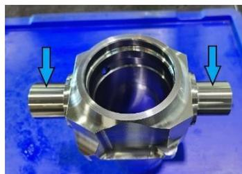
**Gambar 15.** External grinding trunnion
