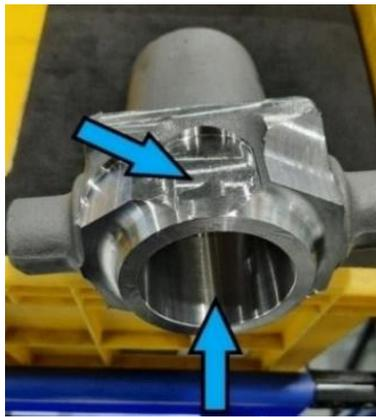
Gambar 8. *Turnmill rough turn and rough mill profile*
