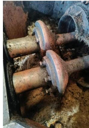
Gambar 3 Adjusting cone
