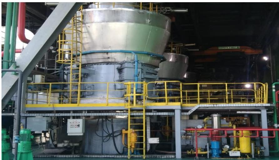
**Gambar 2.** Coal mill (Pulverizer)
