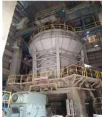
Gambar 7. Vertical raw mill P-10.
