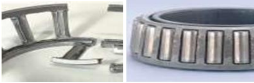
G.16 Failure of cage [3]
