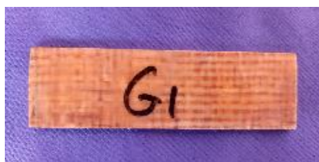
Gambar 2. Spesimen uji water absorption
