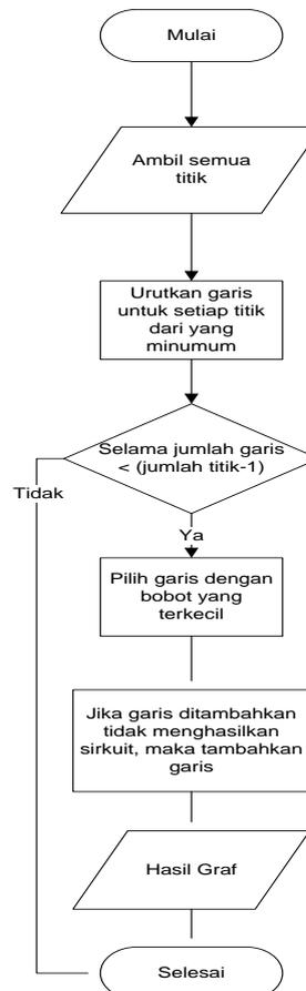
Gambar 4. Diagram Alur Algoritma Kruskal
